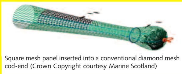
Square mesh panel inserted into a conventional diamond mesh cod-end (Crown Copyright courtesy Marine Scotland)
